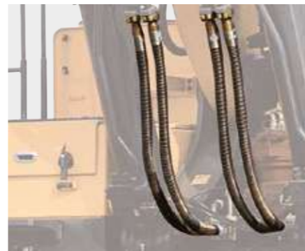
Hydraulic hose High-grade hoses with outstanding resistance to heat and pressure provide maximum durability, even in rough working conditions.
